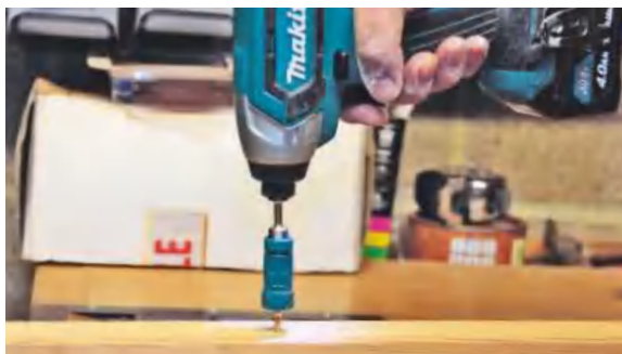
... while the impact driver made 90mm screws bump into softwood with ease
